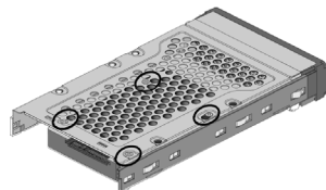
Figure 2-7. 2.5-inch Drive Carrier with 3.5-inch SAS/SATA Drive
