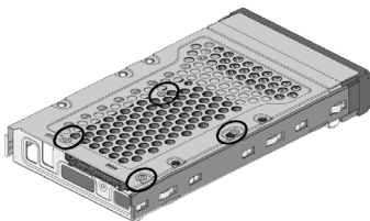
Figure 2-17. Securing Drive
