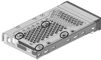
Figure 2-17. Securing Drive
