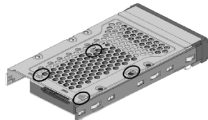
Figure 2-7. 3.5-inch Drive Carrier with 2.5-inch SAS/SATA Drive
