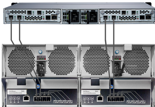
Figure 1-11. Dual Controller Daisy-chain
