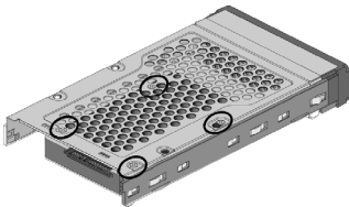
Figure 2-4-1. Installing 2.5-inch SAS/SATA Drive
