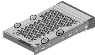
Figure 2-4-2. Installing 3.5-inch SAS/SATA Drive
