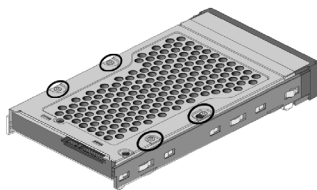
Figure 2-4-2. Installing 3.5-inch SAS/SATA Drive
