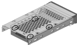
Figure 2-5. 3.5-inch Drive Carrier with 2.5-inch SAS/SATA Drive
