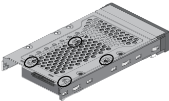
Figure 2-4, Installing 2.5-inch SAS/SATA Drive
