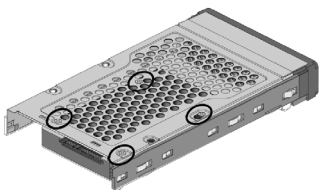
Figure 2-4-1. Installing 2.5-inch SAS/SATA Drive
