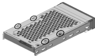
Figure 2-4-2. Installing 3.5-inch SAS/SATA Drive
