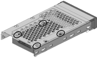
Figure 2-4-1. Installing 2.5-inch SAS/SATA Drive
